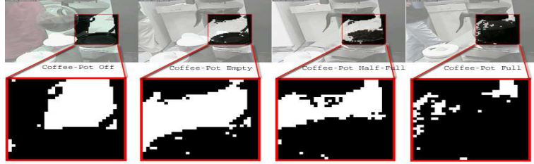
Figure 1. The 4 different states in our example. The black/white cells represent dark/bright average pixel color.
