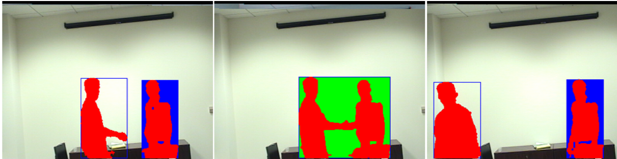
Figure 9. Merging and splitting using the histogram intersection test
