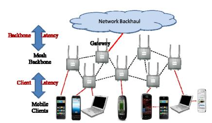
Figure 1: An Instant Mesh Overlay Network
