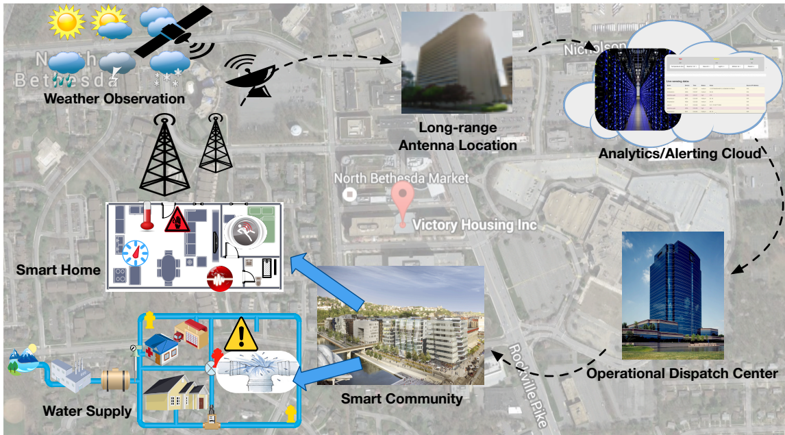
Fig. 1. A general IoT community example with emphasis on water infrastructure. As an example, the cloud constantly collects data from instrumented water meters and seismic sensors via basestations and the regional internet. Based on the analysis of results, a first responder might be dispatched for rescuing.
