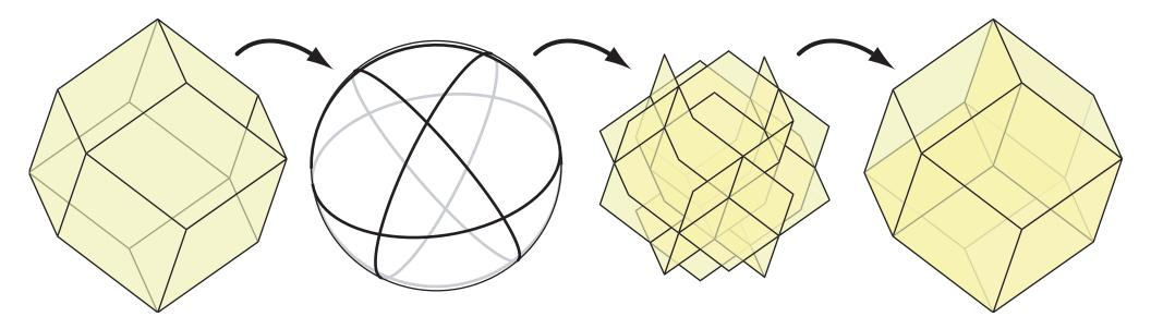
Dualize boundary mesh to curve arrangement on sphere
