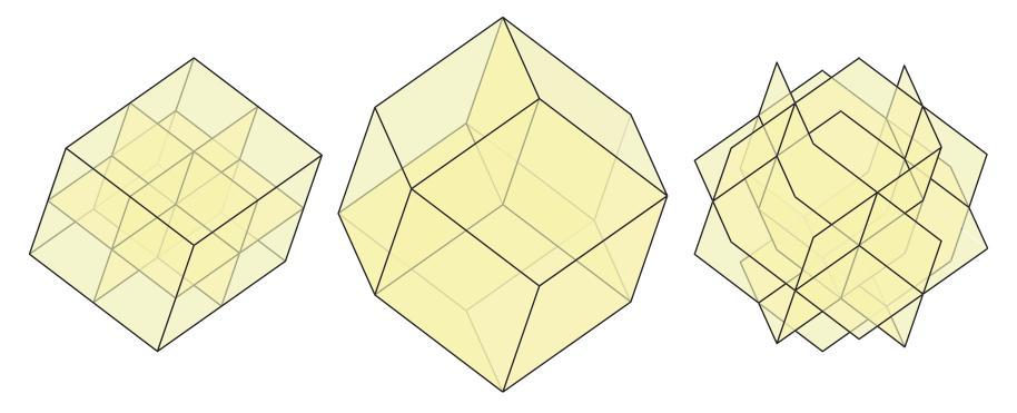
Left: cuboid subdivided by three surfaces into eight pieces Center: four-cuboid mesh of rhombic dodecahedron Right: dual surface arrangement
