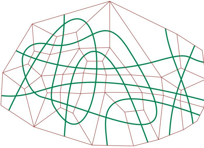
Draw curves connecting opposite edges of each quadrilateral Subdivides quadrilateral into four pieces
