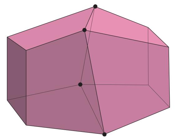
Seems to be the hard case for geometric hex meshing more generally (other domains can be decomposed into bicuboids)
