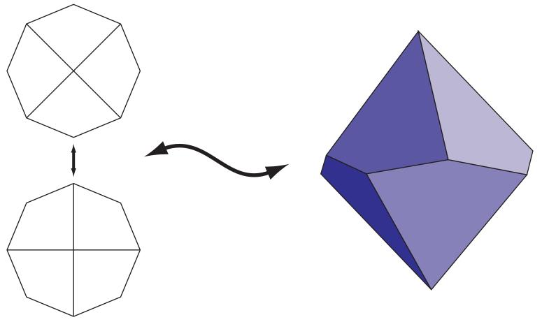
Use a hexahedral mesh to determine set of flips BUT flip sequence ~ shelling, so need shellable mesh
