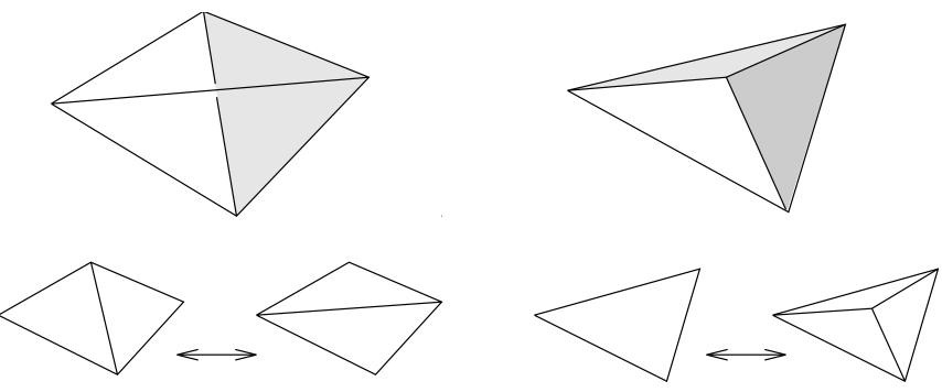
Initial and final configurations of a flip can be viewed as projections of the bottom and top faces of a tetrahedron
