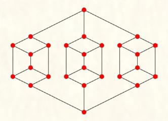
a graph that is NOT a skeleton of a simple orthogonal polyhedron
