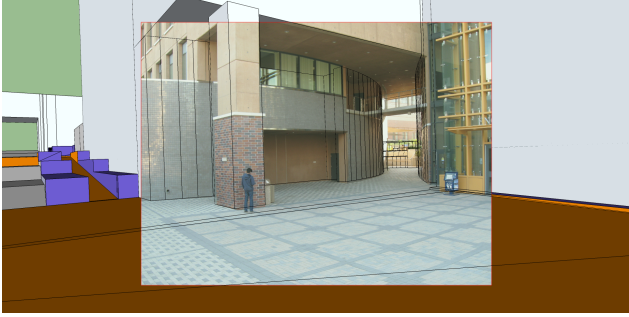
Figure 3: We built a full 3D model from 2D GIS data by creating a toolbox that imports structure from motion reconstruction data into Sketchup. The toolbox allows to read camera information and properly display the image overlaid on the modelling interface. The user then models the 3D geometry by extruding, tilting, and carving the 2D data until it is aligned with the image.
