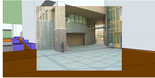
Figure 2: We developed a custom Sketchup plug-in that imports camera parameters computed during bundle adjustment. The user easily models the 3D geometry by extruding, tilting, and carving the 2D map data until it naturally aligns with the image.
