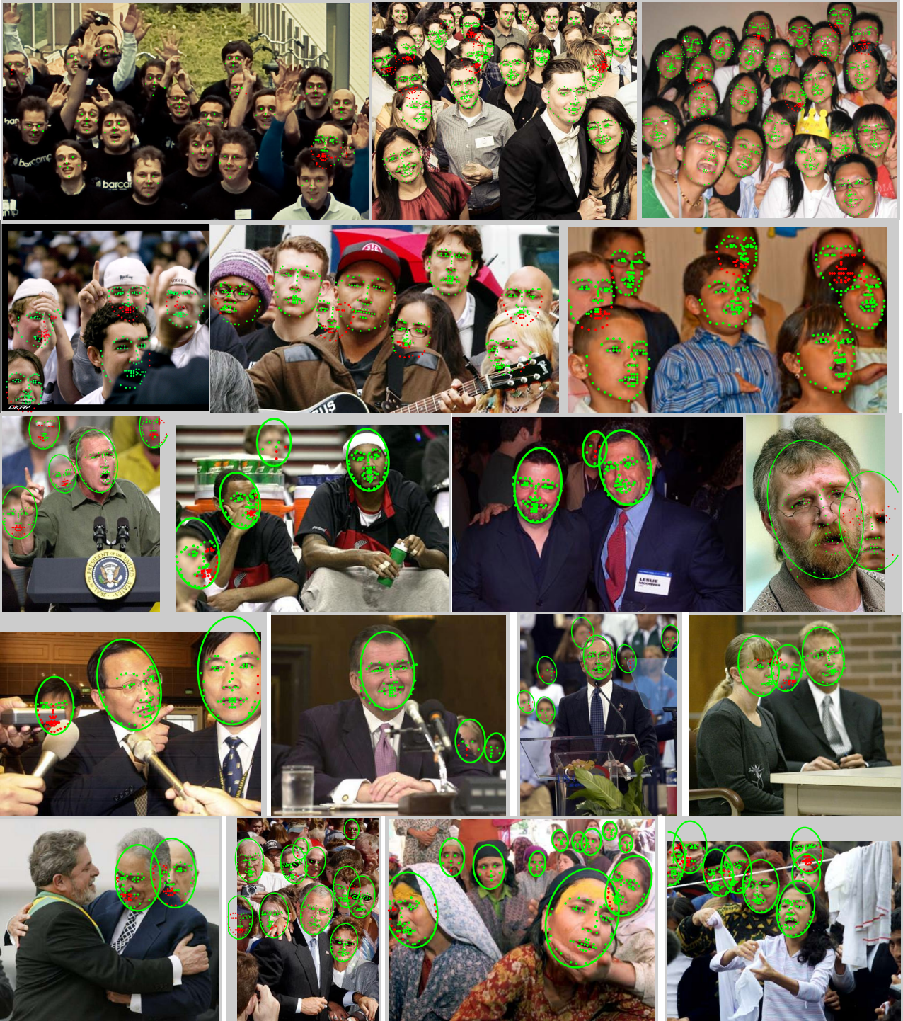
Fig. 11: Examples of detection and localization for images from our UCI-OFD dataset (rows 1-2) and images containing occlusion from FDDB dataset (rows 3-4). Detections indicated with only 7 keypoints correspond to responses from the low-resolution model component. Ellipses are predicted on FDDB images by linear regression from keypoint locations to ellipse parameters.
