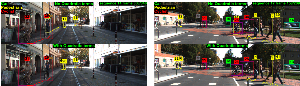
Fig. 1: Our tracking framework incorporates quadratic interactions between objects in order to resolve appearance ambiguity and to boost weak detections. The parameters of the interactions are learned from training examples, allow the tracker to successfully learn mutual exclusion between cyclist and pedestrian, and boost to intra-class co-occurrence of nearby people.
