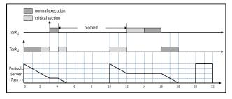
Figure 4: Budget exhaustion inside a critical region with a fixed priority periodic server
