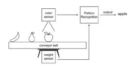
Fig. 2. Pattern recognition based on sensor data collected from items on the conveyor belt.
