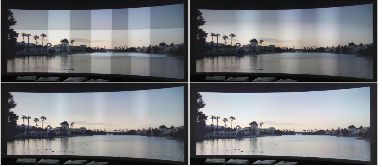
Fig. 6. Comparison of our method with existing work on the most difficult case of white on the curved display made of 2 \times 4 array of eight displays. In scanline order: Before any correction; After simple RGB blending; After applying Majumder and Stevens 2005 photometric seamlessness algorithm with \lambda = 400 ; after our gamut morphing algorithm where the perceptual brightness constraining uses the same method by Majumder and Stevens 2005 with \lambda = 250 .
