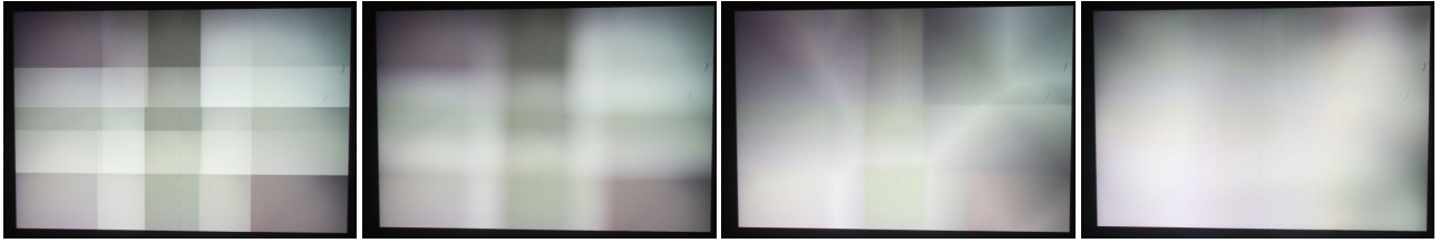
Fig. 5. Comparison of our method with existing work on the most difficult case of white on the planar display. Note that the white is the most difficult test case showing both chrominance and brightness variation. From left to right: Before any correction; After simple RGB blending; After applying Majumder and Stevens 2005 photometric seamlessness algorithm with \lambda = 400 ; after our gamut morphing algorithm where the perceptual brightness constraining uses the same method by Majumder and Stevens 2005 with \lambda = 250 . Please zoom in to see details.
