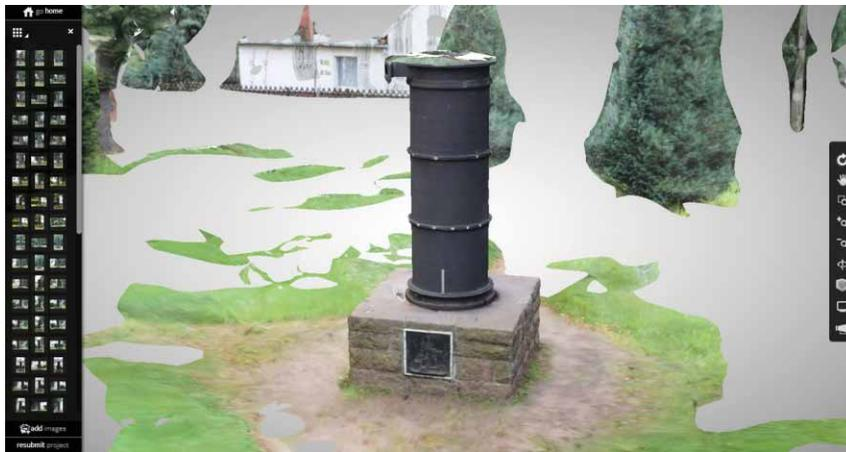
**FIGURE 4.** 3D scene of the Löbejün monument in Photo. The scene represents a triangular mesh of 5.63 million triangles. Users can view a generated mesh at reduced resolution before exporting it as a .rcm, .obj, .fbx, .rcs, or .ipm file.
