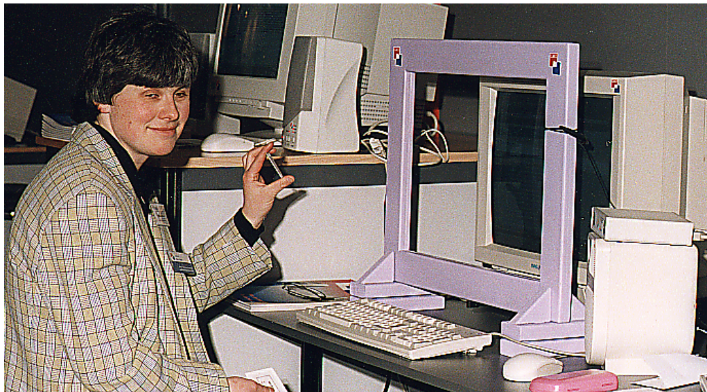
Figure 1: Automatic screen magnification for a mildly vision-impaired user after reading the user profile on the smartcard from a distance
