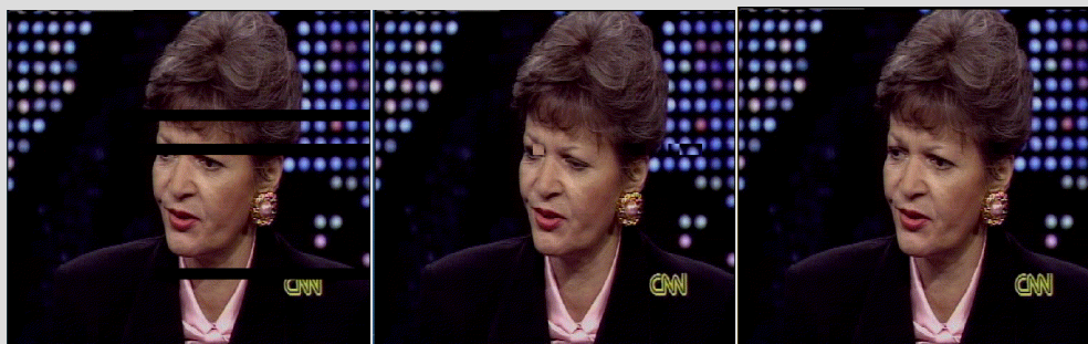
Left: Unconcealed Image. Middle: Concealed by simple motion vector estimation simply averaging the top and bottom mv's. Right: Concealed with more motion vectors. All the adjacent mv's are used directly or indirectly.
