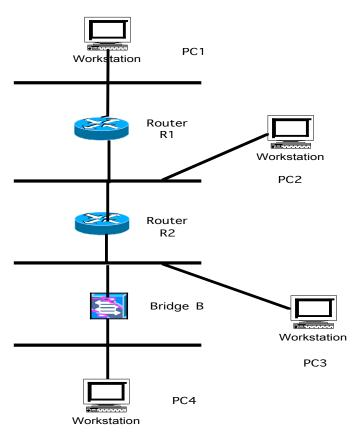
Four PCs are connected to 4 LANs (one PC per LAN). One bridge and 2 routers are used to interconnect the 4 LANs. The campus network address is: 165.143.0.0/16
