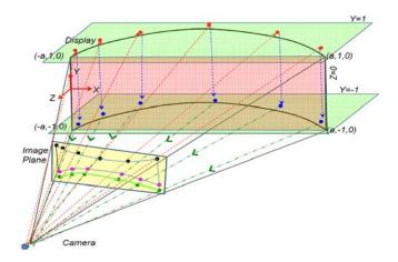
Figure 3: A curve is fitted through the sampled points on the 2D bottom curve (purple line). The sampled points on the 2D top curve in the camera (black) are reprojected in 3D to estimate the 3D top curve (red), and translated down to estimate of the 3D bottom curve (blue), and finally projected back on the camera (green). The distance between these points and the purple curve is minimized in the curve based optimization step.
