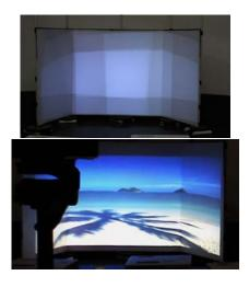
Figure 10: Top: A picture of our CAVE setup with the projectors overlapping on the edges. Bottom: Geometric registration on our CAVE setup. The calibrating camera is visible in the top-left corner of the picture.
