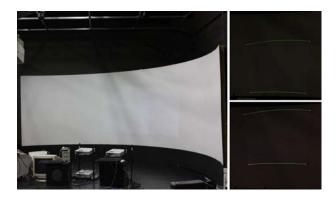
Figure 1: Left: The image  $I_0$  used for estimating camera and display properties. Right: The zoomed in view of  $I_1$  and  $I_2$  for one of our setups, where the projector 1 and 2 are projecting the single pattern used for auto-calibration.
