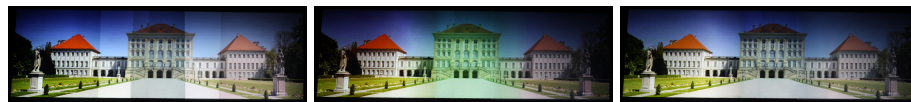
Fig. 7. Color uniformity on a display made of 3 heterogeneous projectors (LCD, LCoS and DLP from left to right): Before any color matching (left), after color matching using ideal devices method (middle) and our method (right). Note that the method for ideal devices introduces a color mismatch in the middle projector by changing the color temperature. Our method balances the brightness better, making the left projector of comparable brightness as the other two. Please zoom-in to see the differences.
