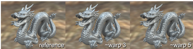
Figure 11: Application of visual equivalence predictors to the Lightcuts rendering algorithm. Using a warp3 based error threshold reduced the rendering time in half, while the warp5 based threshold was correctly predicted as not acceptable.
