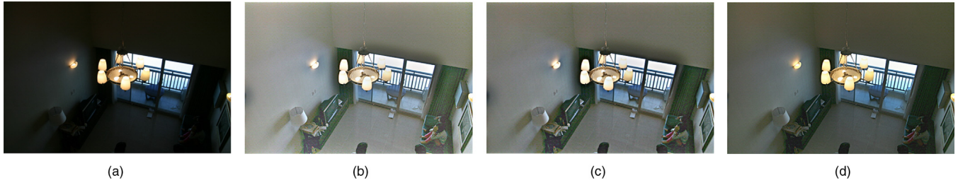
Figure 21. (a) Veranda image, and images resulting from (b) conventional multiscale retinex, (c) proposed color correction, and (d) proposed color correction and chroma compensation.
