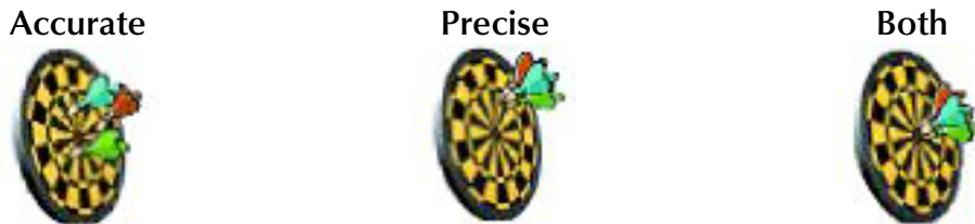
Figure 16: An illustration of precision and accuracy using a dartboard.
