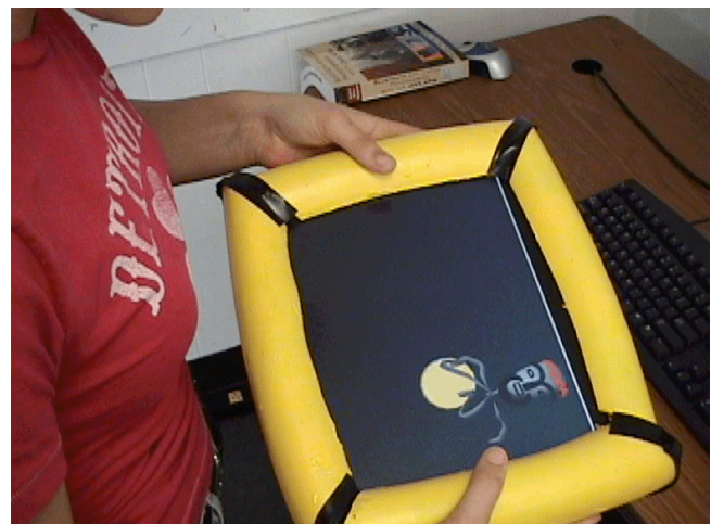
Figure 2: The raft may be used to carry the character to other islands. While on the raft, the character reacts to the physical motion of the device.
