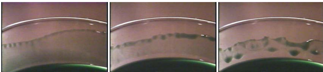
Fig. 4 Alcohol in wine evaporates more at top causing surface tension to be greater at the top of film on the side of the glass. This pulls wine up accumulating at the top forming "wine tears"
