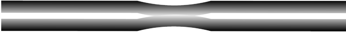
Fig. 3 In a liquid film the surface energy (surface tension) decreases where the surface phases overlap
