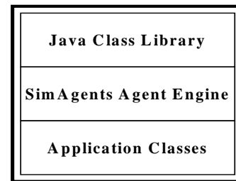
FIGURE 4. Object hierarchy of AgentEngine to Java Class Libraries and Application Classes
