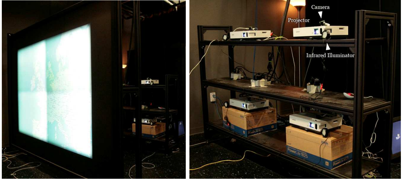
Figure 5: Our setup for the large dataset visualization with back projection system including four PPPs.
