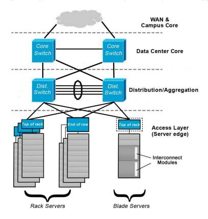
Figure 1: A typical data center structure today uses three layers: access, aggregation, and core.
