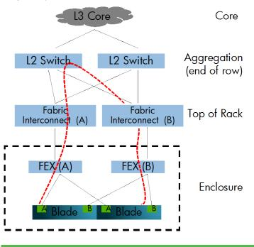
Figure 4: Port extension technology adds an extra "hop" to the typical three-tier architecture and can magnify congestion problems.
