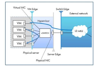
Figure 5: vSwitches do a good job of efficiently routing internal VM-to-VM traffic.
