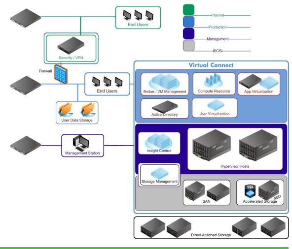
**Figure 3:** When using a VDI configuration Virtual Connect technology, only a small amount of production (protocol) and management traffic exit the Virtual Connect domain, thus optimizing the E/W traffic flow.
