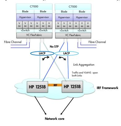
Figure 8: HP IRF technology can combine with Virtual Connect technology to flatten the L2 network.
