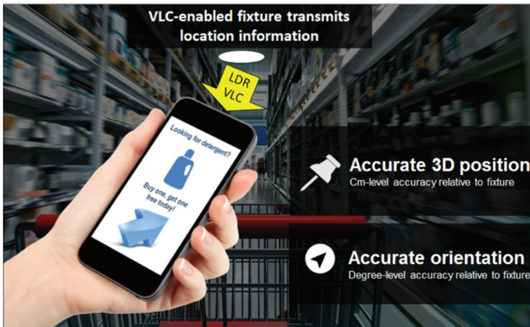
Figure 6. Low Data Rate (LDR) Visible Light Communication that uses simple, power-efficient ON-OFF signaling can be decoded by the smartphone camera sensor. Combined with triangulation of multiple fixtures, this can enable high accuracy indoor positioning and orientation estimation of mobile devices. This technology is of particular interest to the retail industry as it could enable accurate product search, targeted advertising and customer analytics.
