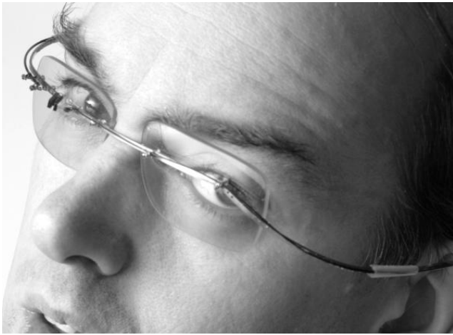
Figure 5: Fully functional electronic eyeglasses built into wire frames. Eyeward-bound light is diverted along the right temple by way of a fiber bundle, into a miniature camera. A laser directs light along another fiber system on the left temple to redraw the modified reality onto the retina. The details are provided in [7].
