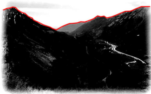
Figure 3: Horizon shapes extracted from a visual scene can be used statically to look up the observer’s location from a prebuilt dataset or dynamically to compute movement of the vehicle mounted camera.
