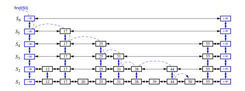
Figure 0.1: Example of a skip list. The dashed lines show the traversal of the structure performed when searching for key 50.
