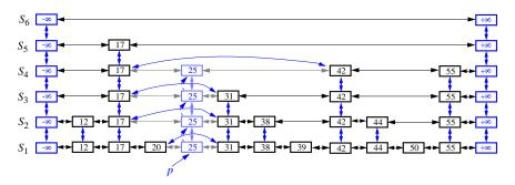
Figure 0.2: Removal of the item with key 25 from a skip list. The positions visited are in the tower for key 25.
