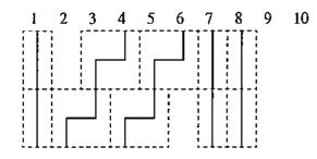
The first and third phases consist of the same operation: routing wires without crossing or branching. The second phase is an even simpler process of copying values into adjacent columns to the right. We describe its operation first.
