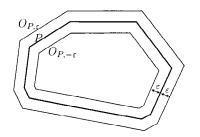
Fig. 1. Inner and outer  $\varepsilon$ -offsets of a convex polygon.
