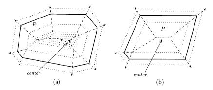
Fig. 2. Offset of a convex polygon based on its medial axis. (a) Point center and (b) segment center.
