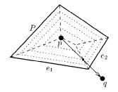
Fig. 3. Dominating edges for the convex polygon-offset distance function.
