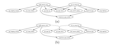
Figure 3: A call graph (a) and its confluent drawing (b), with the dashed part showing the confluence.
