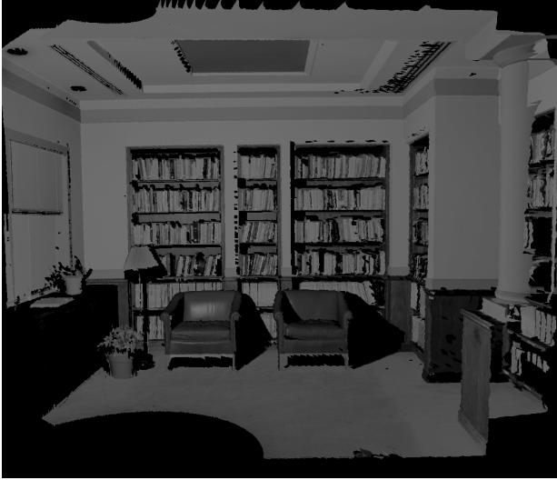
Figure 4: Organized, noisy, massive range data set with 6.48 million points, 143858 points retained, 267131 triangles, 88.5 seconds to reconstruct.
