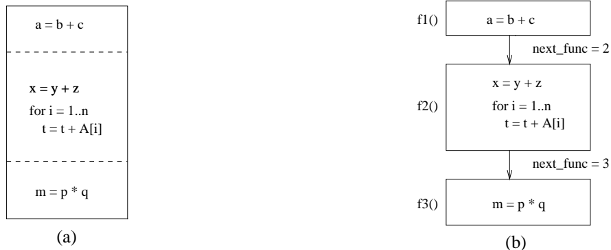
Fig. 7. Mechanism for run-time migration. (a) MESSENGERS code. (b) Translated functions.
