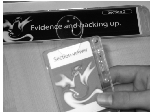
Figure 5. Triggering a transition in the GUI by placing the ‘section viewer’ on the activity square.
