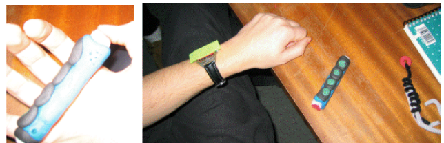
Figure 4. A three part mobile phone interface: a watch display, earpiece (prototyped with pipe-cleaners), and a hand held keyboard. The keyboard is voice activated, and has four keys which permit chording and a select button on the thumb.
