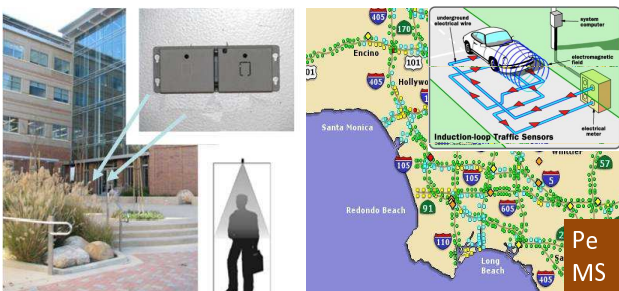
Fig. 1. The left panel shows an optical people counter that we installed at the CalIT2 building on UCI's campus. Loop detectors maintained by the California Department of Transportation on Southern California freeways are shown in the right panel (measurements obtained via PeMS). Sensors such as these report measurements of human activity in real-time.
