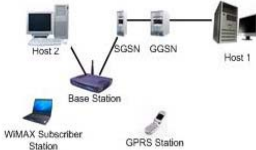
Figure 5 The topology of the simulated GPRS/WiMAX coexistence network.
