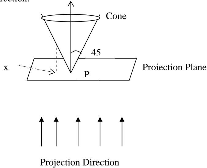
The surface of the cone makes an angle 45 degrees with the axis of the cone. The axis is parallel to the projection direction, and the apex (P) is on the projection plane. Assume that you are drawing the cone (and not the projection plane). What will be the depth value at any arbitrary point x on the plane? Express it in terms of distance(x, P), which is the distance between point x and P. [5]
