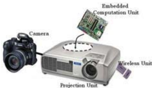
Figure 1: A Plug-and-Play Projector (PPP) consisting of a camera, a projector, and a processing unit.
