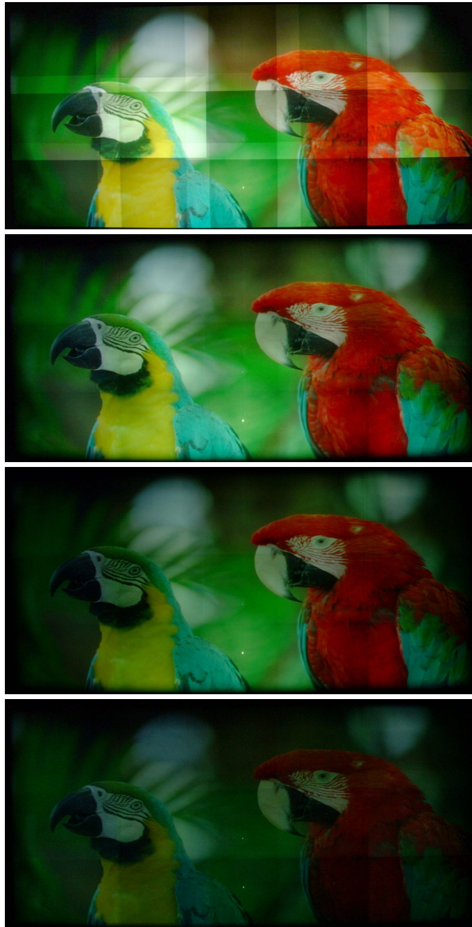
Fig. 7. Digital photographs of a fifteen projector tiled display ( 8' \times 10' in size) before any correction (top), after constraint gradient based smoothing with smoothing parameter of \lambda = 400 , (second from top) \lambda = 800 (third from top) and after photometric uniformity i.e. \lambda = \infty (bottom). Note that the dynamic range of the display reduces as the smoothing parameter increases. At \lambda = \infty is the special case of photometric uniformity where the display has a very low dynamic range.
