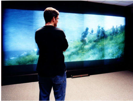
Fig. 14. The correction applied to a non-Lambertian screen and viewed from a view direction that makes an angle of less than 20 degrees with the screen.
