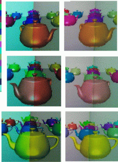
Fig 1 : The different steps of the method on an abutting pair of nView and SONY projectors. Left to right : Before any correction, After non-linearity correction, After luminance correction, After chrominance correction.
