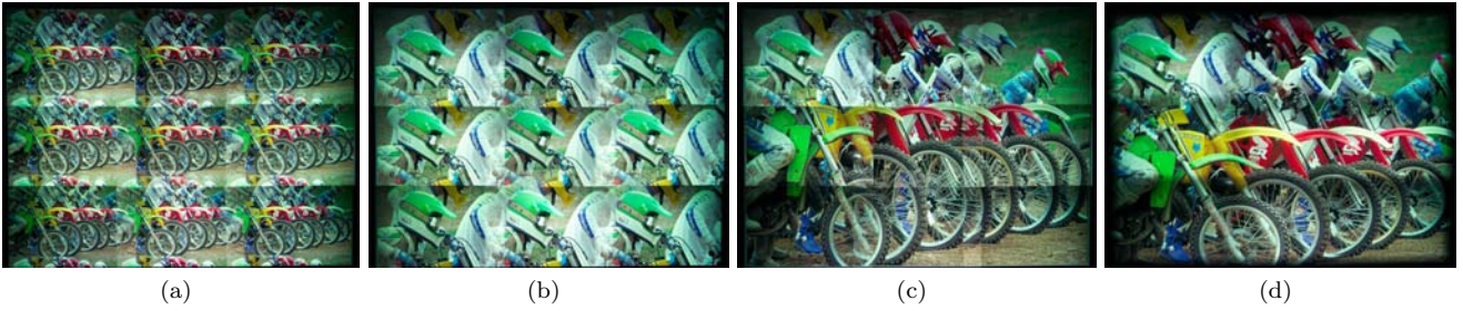
Figure 3: A multi-projector display made of 9 PPPs, if allowed to project data (a) at power on would display the entire data since it thinks it is lone display unit responsible for data display; (b) at the beginning of Configuration Identification process when it is aware that other PPPs would share the responsibility of data display, but thinks that it’s position is (1, 1) and would display the first 1024 \times 768 part of the image; (c) after Configuration Identification step would display the right part of the image, but geometrically and photometrically uncalibrated; and (d) finally, after Alignment would project the seamless image. (d) is the only image that the user would see, rest are used for illustration.
