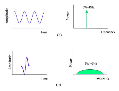
Figure 1. (a) Conventional narrowband communications send long continuous waveforms and generate very narrow frequencies. (b) UWB communications send extremely narrow pulses and generate very wide frequencies.
