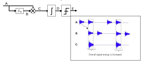
Figure 2: (Left) Block diagram of a multipulse receiver (similar to Fig.2). Dn is the delay between the transmitted pulses. (Right) Signal representation of multipulse receiver in multipath channels. Due to passing through the same channel, the signal energy for correlation is stronger.
