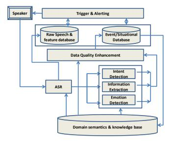
Figure 1. Components of the envisioned Observational Speech System (OSS)
