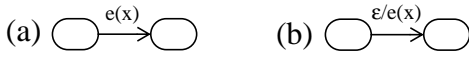
Figure 7. (a) A CSP event with input data, e?x , is modeled in UML State Machines as a state transition event with no action. (b) A CSP event, e , with output data, e!x , is modeled as a null state transition event that results in action e .
