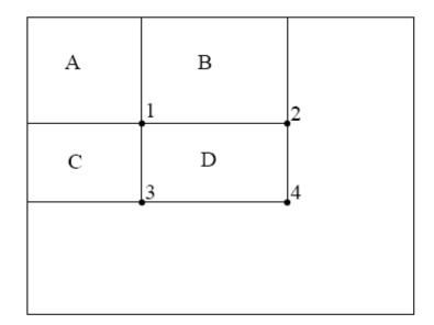
Figure 3: The sum of the pixels within rectangle D can be computed with four array references. The value of the integral image at location 1 is the sum of the pixels in rectangle A. The value at location 2 is A + B, at location 3 is A + C, and at location 4 is A + B + C + D. The sum within D can be computed as 4 + 1 - (2 + 3).
