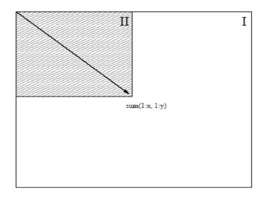
• A representation that means any rectangle's values can be calculated in four accesses of the integral image.
