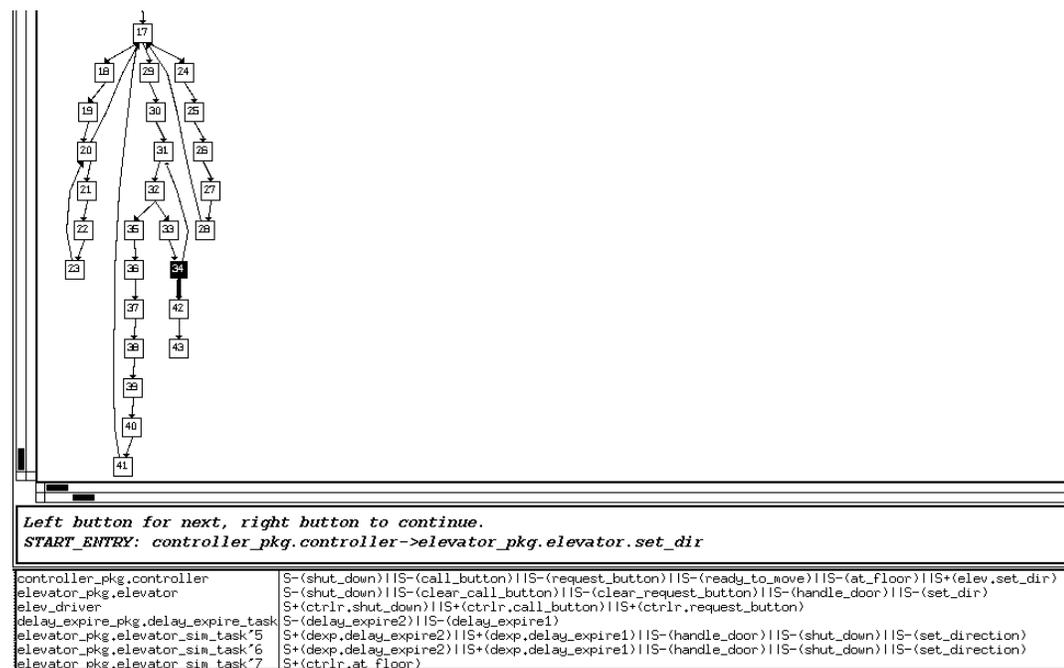
Figure 4.3: System output for failed execution of elevator. The graph at top shows a portion of the TICG built from the trace. The text box immediately below gives a description of the highlighted task transition which led to failure. The bottom shows the task state window which contains the state from which the failed transition occurred.
